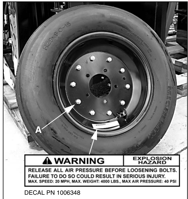
Figure 28. Split Rim Tire Servicing
